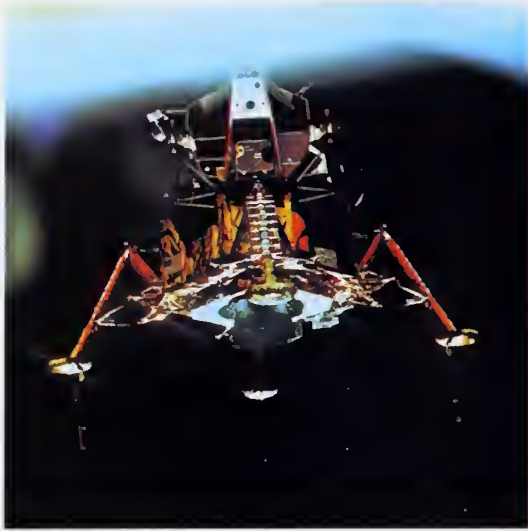
Apollo 11 Lunar Module with its four landing-gear footpads deployed for touchdown. This photograph was taken from the Command Module as the two spacecraft moved apart above the Moon on July 20, 1969.
